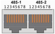
With dual RS485 interfaces, the default baud rate is 19200bps. If you need to communicate the batteries in parallel with the monitoring device or inverter, you need to connect each battery with RS485-1 and RS485-2 ports, so the host battery can read the information of each battery.
