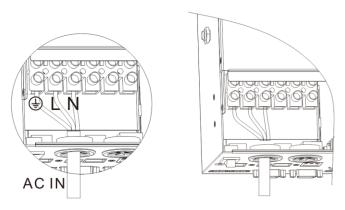
③ Correctly connect AC output wire in accordance with cable sequence and terminal position shown in the figure below. Please connect the ground wire at first, and then live wire and null wire. The ground wire is connected to the ground screw hold through Oshaped terminal.
